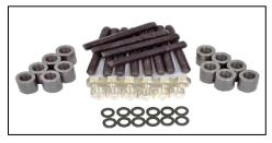
**C13 Exhaust Stud Kit - MCBC13ESK** This new kit is assembled to fit Caterpillar® C11 & C13 models with low turbo charger mounting or low cab forward chassis. The kit contains all the made in the USA hardened studs, locknuts, washers and spacers needed to mount the exhaust manifold.
